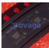
HMC3653LP3BE Analog Devices, Inc QFN-12
