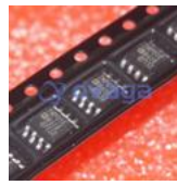
TMP01ES Analog Devices, Inc SOP8
